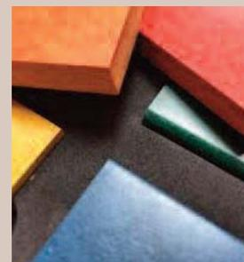
Valchromat is a decorative wood-fibre panel product which is coloured throughout. The fibres are coloured individually, impregnated with organic dyes and bonded together by a special resin giving Valchromat its unique physical and mechanical features. It is an evolution of MDF (Medium Density Fibreboard) and is superior to coloured MDF.
